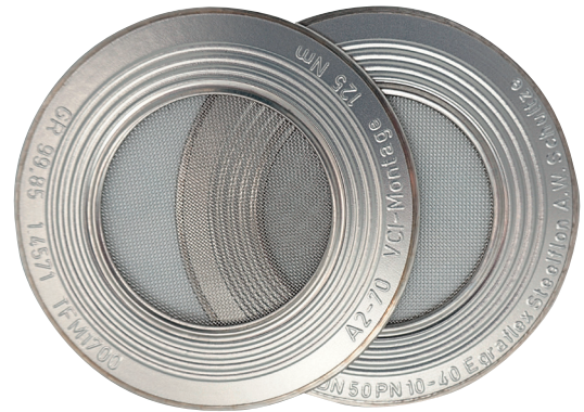
Photo: Push-in sieve – carrier material Egraflex Steelflon with patented refinement process Waveline WLP® for flange with indication of dimensions, material, torque and manufacturer on both sides of the external edge
