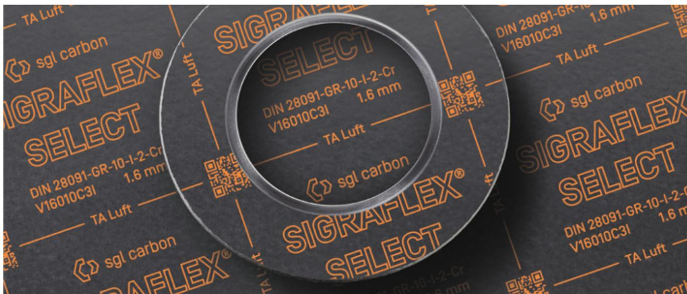
SIGRAFLEX SELECT is a gasket comprised of three SIGRAFLEX flexible graphite foils of various thicknesses reinforced with two 0.05 mm thick stainless steel foils using our proven SIGRAFLEX HOCHDRUCK technology. This gasket has an inner eyelet and is antistick impregnated to reduce leakage and improve handling.
